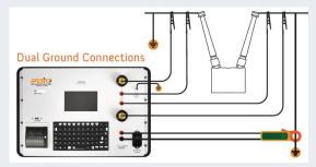
As the rise and fall time is configurable for each test, no transients are induced in the associated apparatus such as current transformers. This avoids maloperation of the connected relays to the current transformers.
